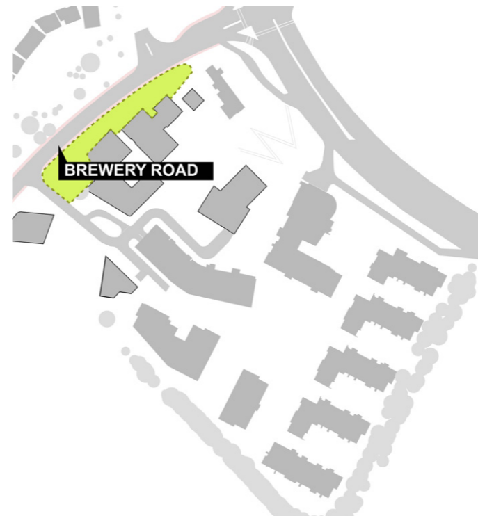
Brewery road A soft landscaping is added along the brewery road. Provides screening for private balconies.
